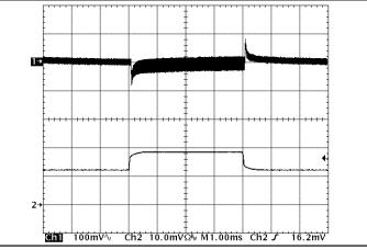
Figure 11: Output voltage response to step-change in load current (50%-75%-50% of lout(max);  $dI/dt = 0.1A / \mu s$ ). Load cap: 10  $\mu$ F, 100 m $\Omega$  ESR tantalum cap and 1 $\mu$ F ceramic cap. Ch 1: Vout (100 mV/div). Ch 2: lout (10 A/div).
