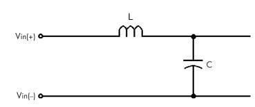
Figure E: Internal Input Filter Diagram (component values listed on the specifications page).
