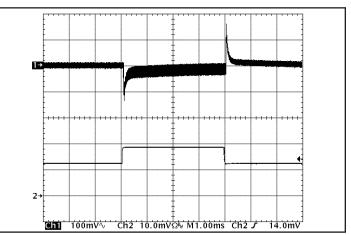
Figure 12: Output voltage response to step-change in load current (50%-75%-50% of lout(max):  $dl/dt = 5 A/\mu s$ ). Load cap: 470  $\mu F$ , 30 m $\Omega$  ESR tantalum cap and 1  $\mu F$  ceramic cap. Ch 1: Vout (100 mV/div), Ch 2: lout (10 A/div).
